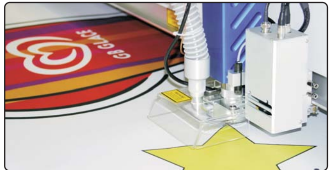
Laser cutting of printed materials by camera recognition
