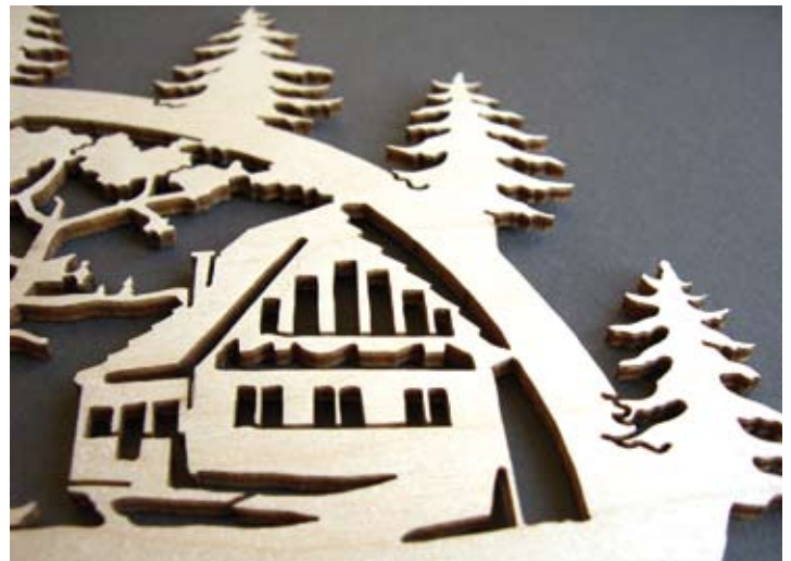
Extremely fine contours due to contactless cutting
